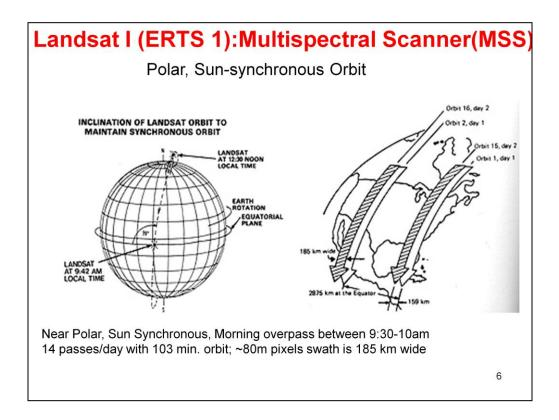
The first one to three Landsats orbited at an altitude of 570 miles (923 km); 4 and 5 at 435 miles (705 km).
