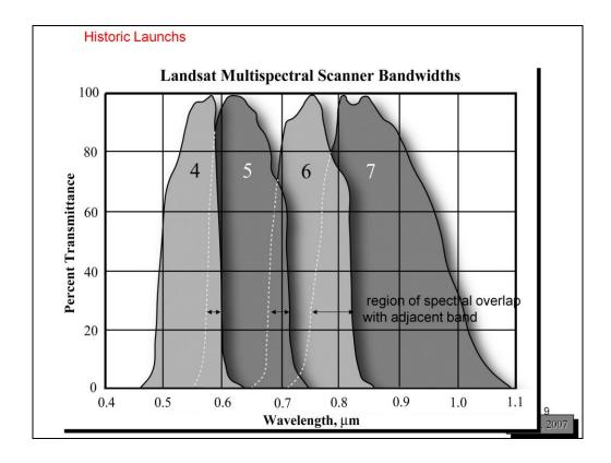
Due to issues with the detector sensitivity and the filters used in fabricating the detector, band passes do not have non-overlapping square-wave structure but are sensitive to some wavelengths more than others and some wavelengths are detected by more than one band.
