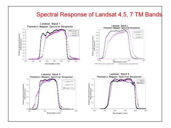
As the instruments in a series evolve with different versions, the data recorded also changes. This example shows spectrometer differences for recent Landsat TM series 4, 5, 7. Differences between different instruments are significantly greater than this. Thus when someone produces an NDVI or EVI or some other index with different instruments, the differences between instruments may be greater than the actual spectral differences.
