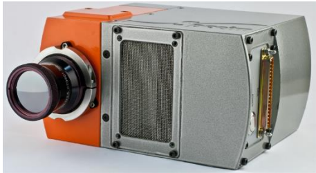
Hyperspectral imager 100s of bands, visible through reflected solar infrared (to 2500nm)
