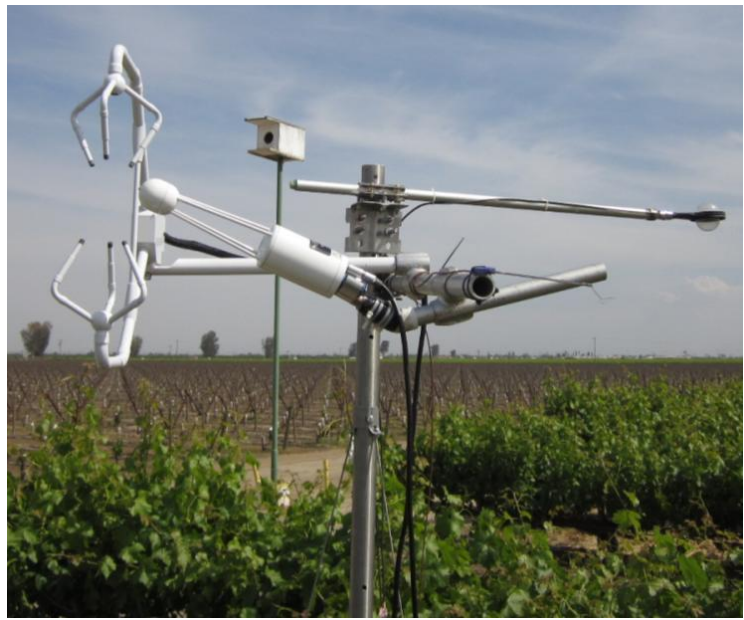
EC System measures gas concentrations, transport rates, and general weather station data
