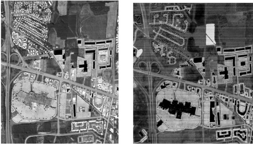
September 1994 Period of maximum heating (solar noon) and shortly after sundown when the heat storage is the greatest.
