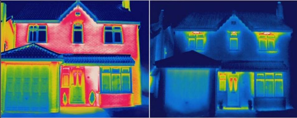
Thermal scans of a house before, left, and after being insulated. In Britain, subsidies cover much of the cost of home insulation.
