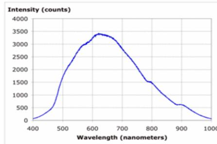
The spectrum of an incandescent bulb in a typical flashlight. Here, the filament temperature appears to be about 4600 K due to a peak emittance around 630 nm. The shape shows that the filament is not a true black body.
