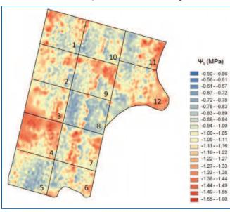
Figure 1. Leaf water potential map of 16 ha of "Chardonnay" vineyard, obtained from high resolution thermal images. Estimated  $\Psi$ L values were obtained from relationship between CWSI and  $\Psi$ L in stage II.
