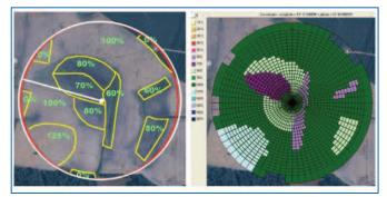
Figure 4. Irrigation application rates assigned to different areas under a 48 ha center pivot irrigation system (left) and variable rate irrigation implementation of the application map (right)
