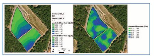
Figure 2: Map of (a) estimated flow rate and (b) measured flow rate.
