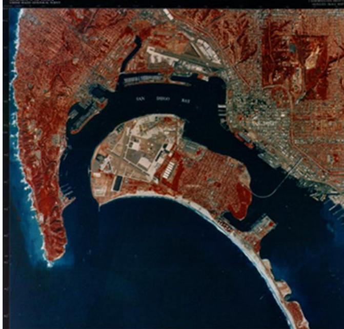
November 22, 1988, SPOT image of San Diego, 3 multispectral HRV bands at 20 m resolution, are combined and registered with the 10 m panchromatic image
