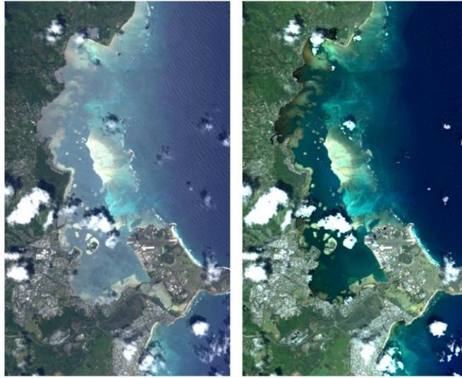
Example of glint correction using subtraction of NIR reflectance. (Left) Original AVIRIS scene of Kaneohe Bay, Hawaii (f000412t01p03\_r08). (Right) The scene after atmosphere and glint correction. Clouds and some sea surface features remain; this is due to automated masking. Overall, glint correction performs quite well.
